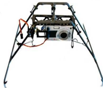
10mp stills (3648x 2736 Pixel) w/ stabilisation, 1GB card, IR trigger & tilt control
